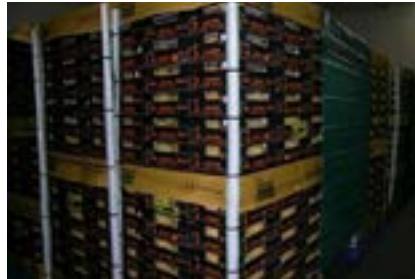
Fig. 5: Large openings at the top center of each side of the carton provide unrestricted air flow across the pallet along both axes.
