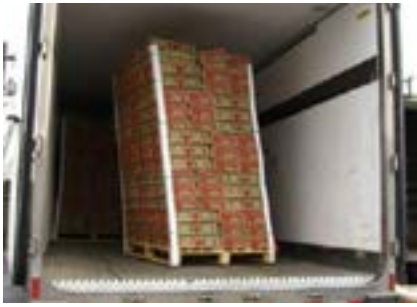
Fig. 4: Pallet cannot support the weight due to weak, poorly designed cartons. The sagging cartons obstruct ventilation and are likely to cause damage to the produce.
